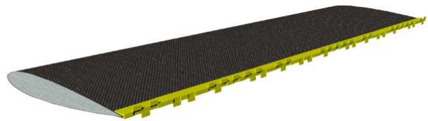
Fig. 1 A perspective view of a conceptual wing with miniature flaps attached to the trailing edge
