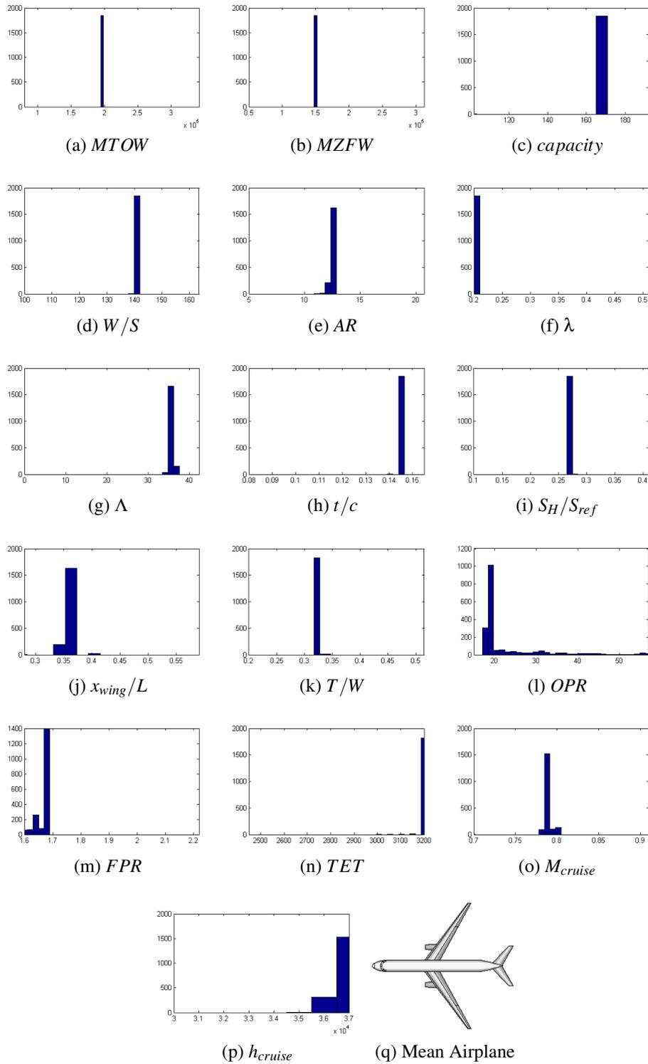
**Fig. 6** Histograms of each airplane design variable and a top view of the mean airplane from the final Pareto front.
