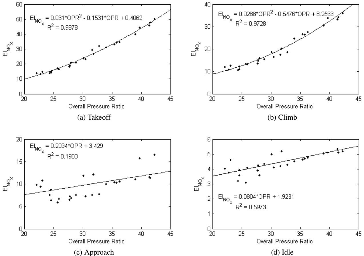
**Fig. 1** Fits of  $NO_x$  emission index at the four certification points as a function of overall pressure ratio.
