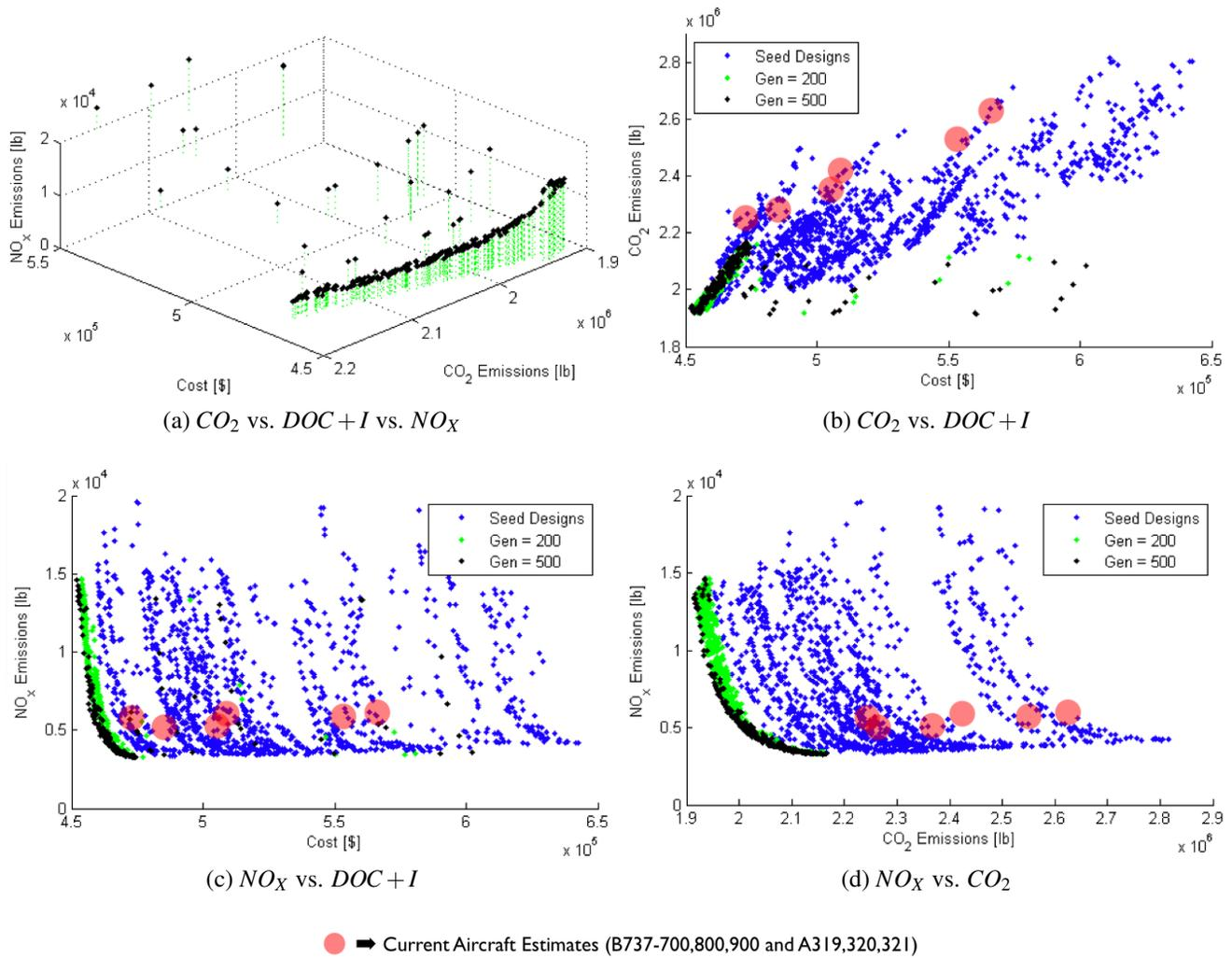
**Fig. 5** The final Pareto front and the projections into the objective planes of the population seeds, the Pareto front at generations 200 and 500, and the estimated performance of current aircraft.
