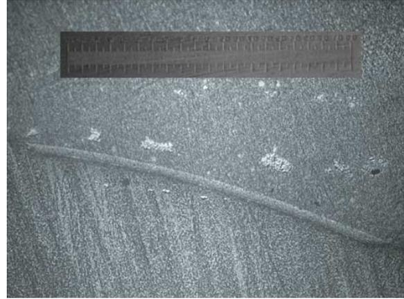
Figure 12. SEM image of section shape at 0.75R. Chord is approximately 3mm.
