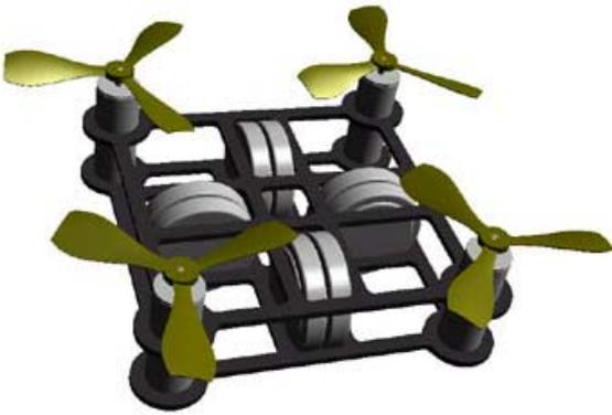
Figure 13. CAD model of multi-cell Mesicopter prototype.
