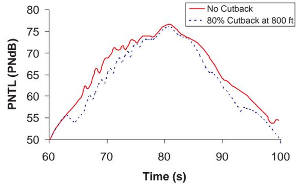
Figure 6: Perceived noise level during simulated flyover of two procedures: without cutback and with 80% throttle cutback at 800 ft.
