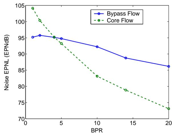
Figure 3: Noise as a function of bypass ratio.
