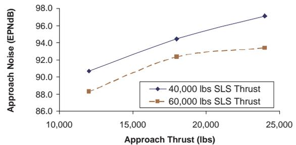
Figure 8: Comparison of the approach noise of 40,000 lbs and 60,000 lbs sea level static thrust engines as a function of approach thrust.
