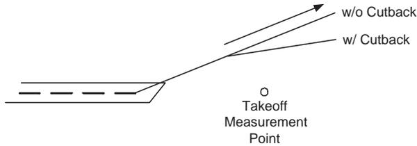
Figure 5: Thrust Cutback on Take-off.
