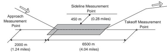
Figure 2: ICAO Noise Measurement Points.
